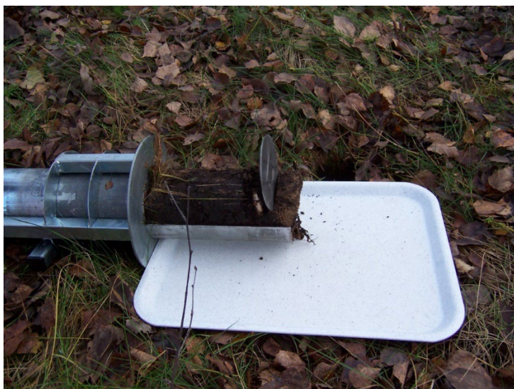
Figure 6. Slicing of a soil sample taken with a golf hole cutter.
