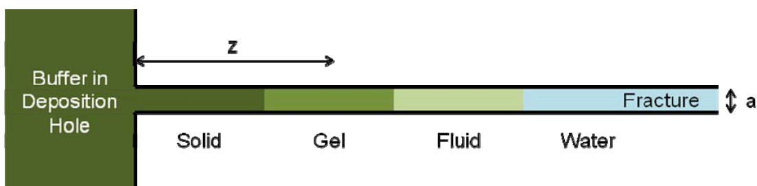
Figure 9. Conceptual model of buffer erosion (from Birgersson et al., 2009). The swelling pressure and density of bentonite in the fracture decreases exponentially with increasing distance, z , and, at a given distance, with decreasing fracture aperture, a .
