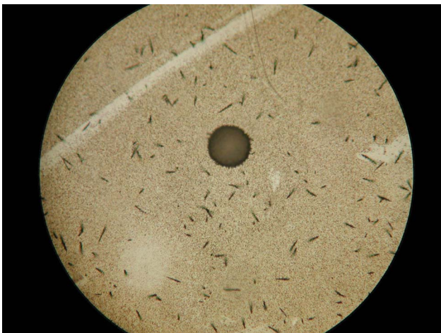
Figure 3. Track-etch prints of a U-oxide particle, ( ^{235}\text{U}/^{238}\text{U} 0,25), NIST sample 3, 500 \times magnification.
