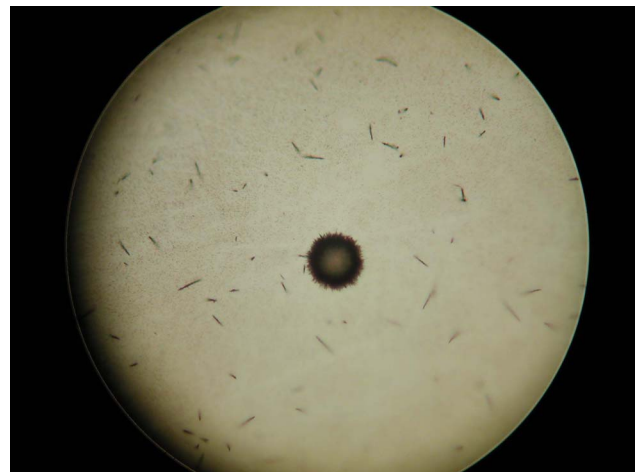
Figure 4. Track-etch prints of a U-oxide particle, ( ^{235}\text{U}/^{238}\text{U} 0,03), NIST sample 4, 500 \times magnification.
