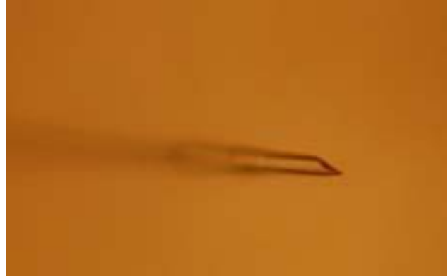
Figure 12. The tip of a capillary under 200 \times magnification.
