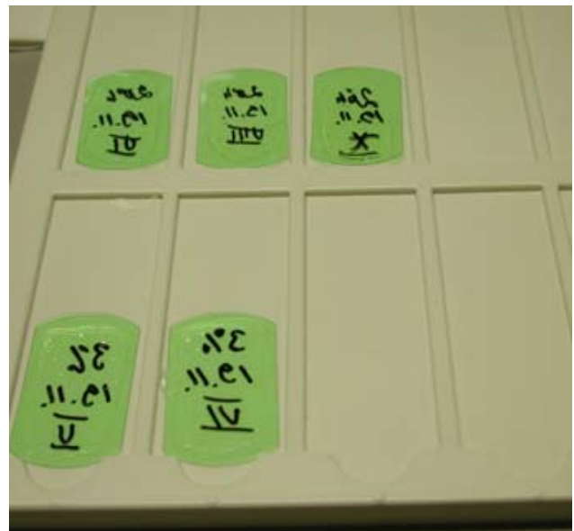
Figure 3. Irradiated Makrofol detectors before etching.
