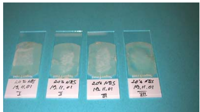
Figure 4. Etched Makrofol glued on microscope slides.
