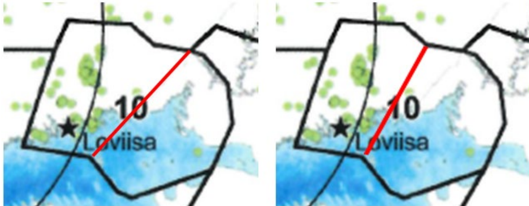
Fig. 3-5. Two alternative designs of the seismic source area no. 10. Available earthquake epicentres (green dots) and the divisions of area source no. 10 by red lines. The excluded area was added to source area 6. The star denotes the NPP site.
