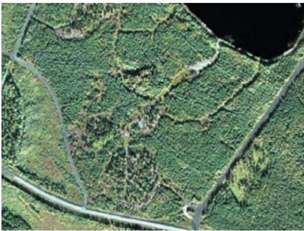
Figure 4. Combination of QuickBird multi-spectral image sharpened with the panchromatic channel from the geographical location of Onkalo. This image (September 9, 2002) includes the near infrared spectral band, which causes light colour of broad-leaved tree forest.
