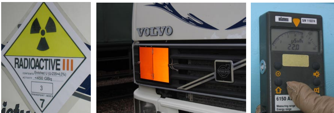
Figure 7. Labelling, placarding and radiation measurements are checked in a transport inspection.
