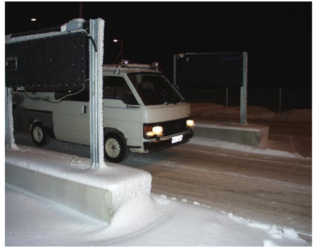
Figure 8. Automatic radiation portal monitor at Raja-Jooseppi border station.
